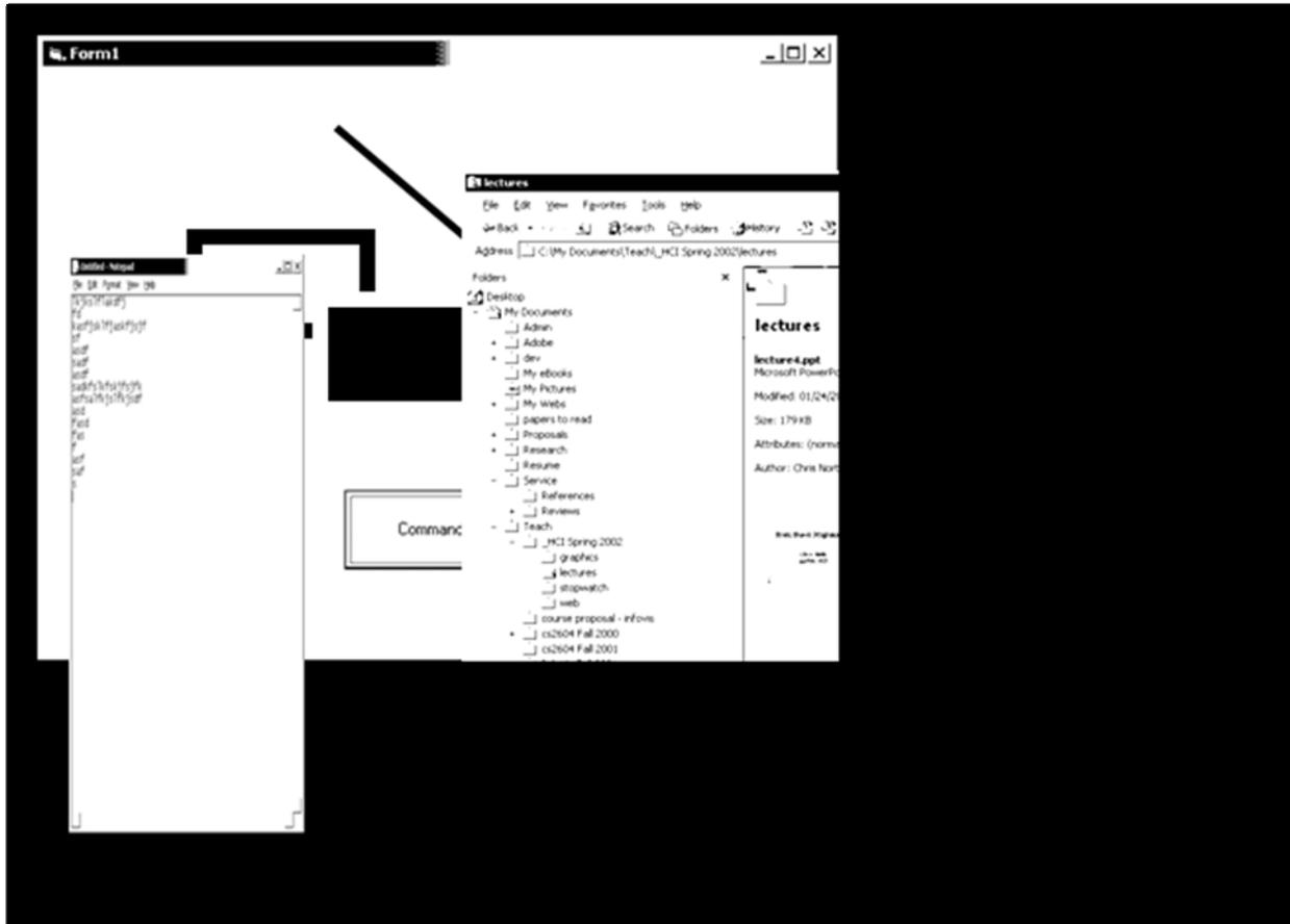
The following figure shows the situation when myApp's JPanel calls its repaint method. Notice that some portion of window explorer is still remains in front of JButton because yet not repaint event is sent to it.
