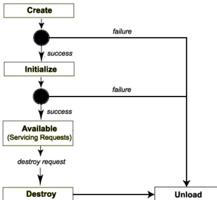
The web sever creates a servlet instance. After successful creation, the servlet enters into initialization phase. Here, `init()` method is invoked for once. In case web server fails in previous two stages, the servlet instance is unloaded from the server.
