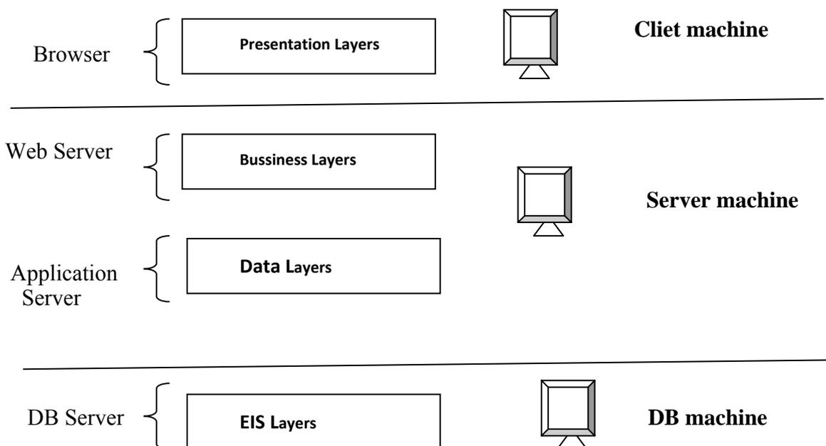
The client tier represents the client machine where actually web browser is running and usually displays HTML. You can think of a Presentation as of two parts; one is on client side, for example, HTML. There is also a presentation layer that is used to generate the client presentation often called *server presentation*. We'll discuss about it later.
