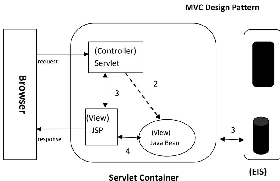
The client (browser) sends all the requests to the controller. Servlet/JSP acts as the *Controller* and is in charge of the request processing and creation of any beans or objects (*Models*) used by the JSP.
