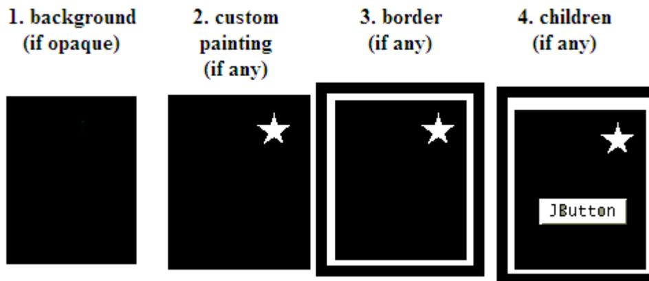
The figure above illustrates the order in which each component that inherits from `JComponent` paint itself.
