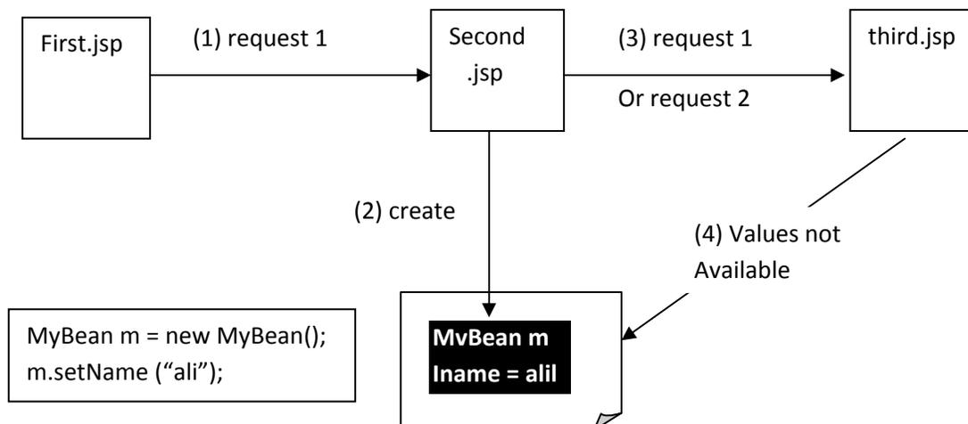
In the diagram above, *first.jsp* generates a request “*request 1*” that is submitted to *second.jsp*. Now, *second.jsp* creates an object *m* of *MyBean* by calling its default constructor and stores a value “*ali*” for the *name* property by making a call to appropriate setter method. Since, the scope specified in this example is “page” when the object of *MyBean* is instantiated using `jsp:useBean` action element. Therefore, object (*m*) of *MyBean* is stored in `PageContext`.
