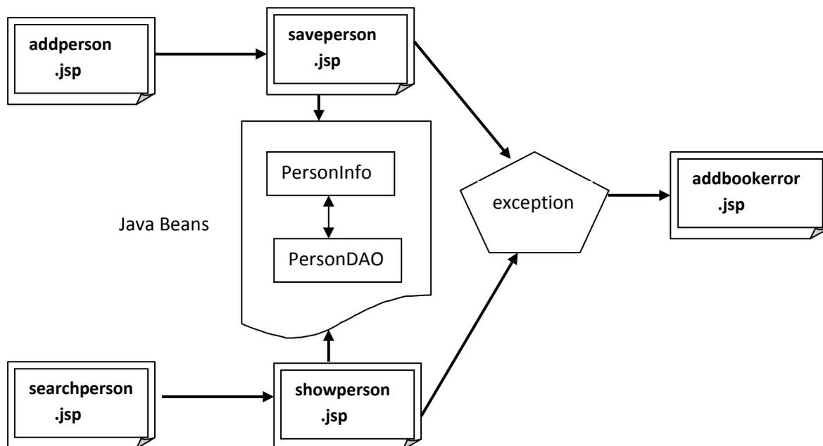
addperson.jsp takes person's information from the user and sends it to saveperson.jsp. After receiving request, saveperson.jsp makes an object of PersonInfo using received information and saves it into the database using PersonDAO Java bean.
