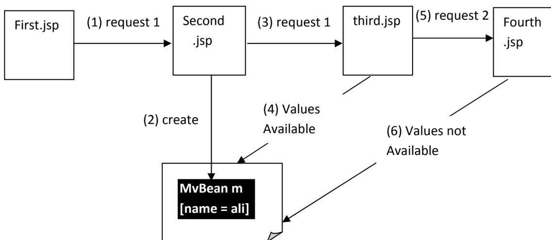
In the diagram above, MyBeans instantiated by specifying scope =“request” that results in storing object in ServletRequest. A value “ali” is also stored in m using setter method.
