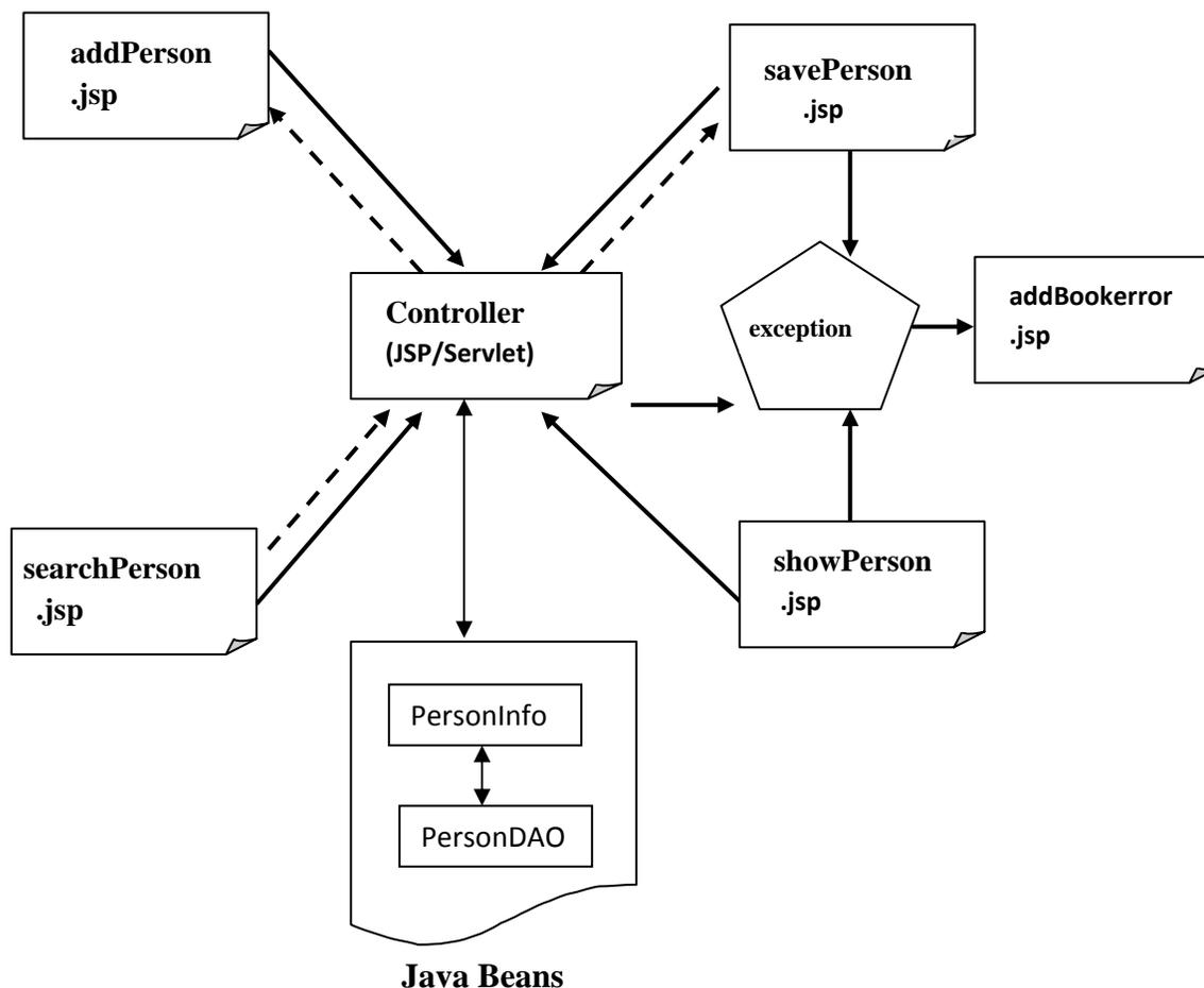
As you can see in the diagram that all the requests are submitted to controller which uses the JavaBeans and forwards/redirects the user to another view (JSP). If any exception arises on controller or JSPs, the control would automatically be transferred to `addBookerror.jsp` to display an appropriate message.
