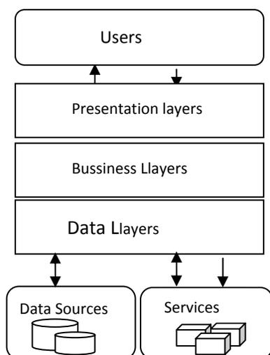
As you can see in the figure, users can only interact with the presentation layer. The presentation layer passes the user request to the business layer, which further passes the request to the data layer. The data layer communicates with the data sources (like Database etc.) or other external services in order to accomplish the user request.
