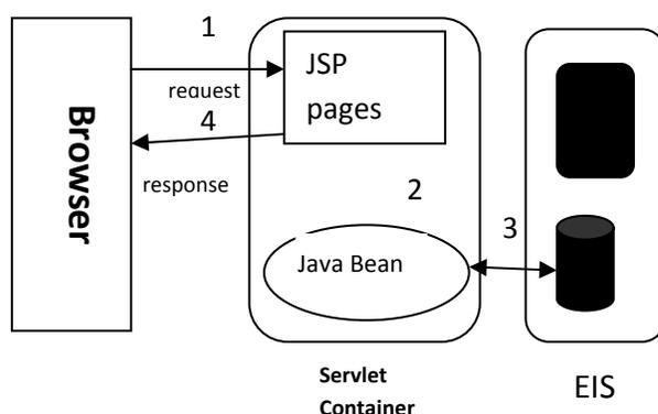
In Model 1 architecture, view selection is decentralized, because the current page being displayed determines the next page to display. In addition, each JSP page or servlet processes its own inputs (parameters from GET or POST). And this is hard to maintain, for example, if you have to change the view selection, then several JSP pages need to be changed. In some Model 1 architectures, choosing the next page to display occurs in scriptlet code, but this usage is considered poor form.
