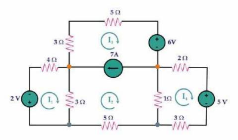
KVL equation for mesh 1 2+4 l1+3 (l1-l2) =0
