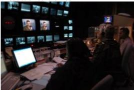
The production control room (also known as the 'gallery') is the place in a television studio in which the composition of the outgoing program takes place. Facilities in a PCR include:
