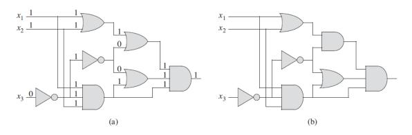
Two instances of the circuit-satisfiability problem. (a) The assignment  $\langle x_1 = 1, x_2 = 1, x_3 = 0 \rangle$  to the inputs of this circuit causes the output of the circuit to be 1. The circuit is therefore satisfiable. (b) No assignment to the inputs of this circuit can cause the output of the circuit to be 1. The circuit is therefore satisfiable.
