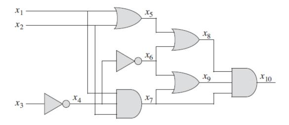
Reducing circuit satisfiability to formula satisfiability. The formula produced by the reduction algorithm has a variable for each wire in the circuit.
