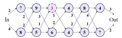
$$\begin{split} f_1[j] &= \min \left( f_1[j-1] + a_{1,j}, \, f_2[j-1] + t_{2, \, j-1} + a_{1,j} \right) \\ f_2[j] &= \min \left( f_2[j-1] + a_{2,j}, \, f_1[j-1] + t_{1, \, j-1} + a_{2,j} \right) \\ j &= 3 \\ f_1[3] &= \min \left( f_1[2] + a_{1, \, 3}, \, f_2[2] + t_{2, \, 2} + a_{1, \, 3} \right) \\ &= \min \left( 18 + 3, \, 16 + 1 + 3 \right) \\ &= \min \left( 21, \, 20 \right) = 20, \end{split}$$
