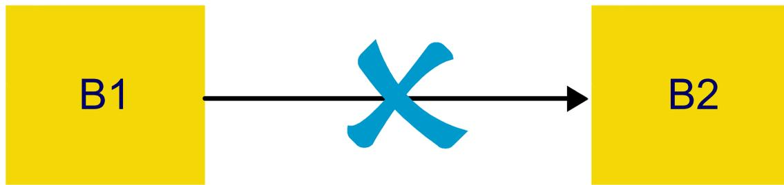
There must be an intermediate process which should transform data received from one external entity and then send the transformed data to the other external entity. As we have already described that data flow diagrams should be used to depict processes that transform or process data. Simple data movement from one entity to another should not be described using data flow diagrams.
