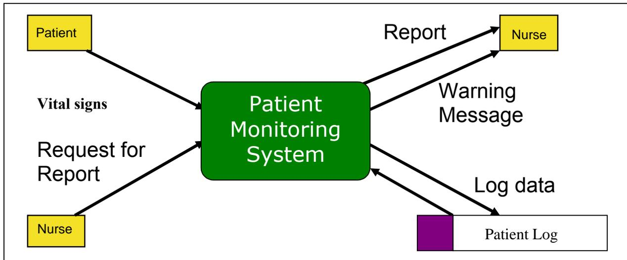
In order to see detail processes involved in Patient Monitoring System, a level 1 data flow diagram will have to be made. In the following, we are providing level 1 data flow diagram which is a refinement of the level-0 data flow diagram.
